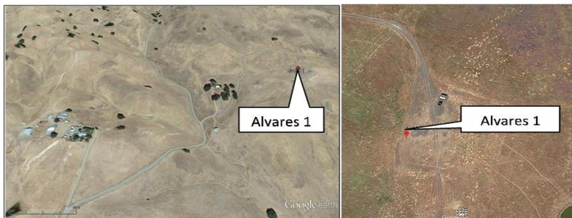
Fig. 1: Alvares location in open ranchlands; more detailed image on the right shows that the original 1982 drilling pad is still evident, and can be restored for planned re-entry
