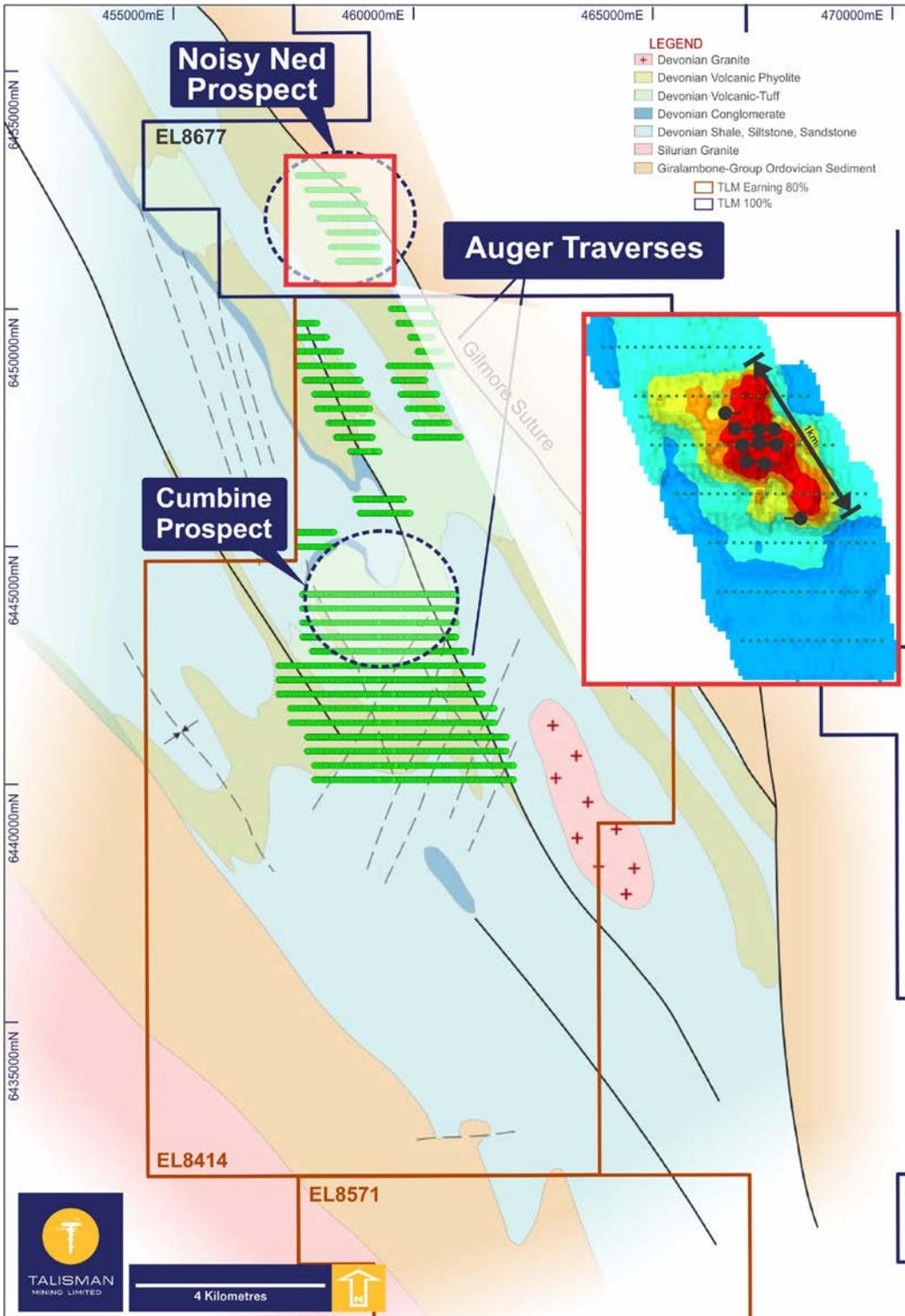
Figure 2: Noisy Ned Prospect - geochemical anomaly showing planned drill collar locations
