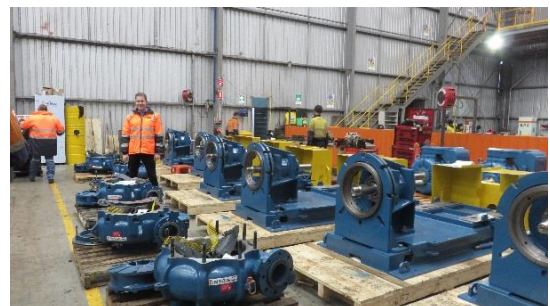
Centrifugal pumps final assembly in workshop
