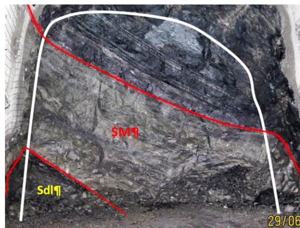
535 ore drive (4.5m W x 4.5m H) with a face grade of 5.7% Ni
