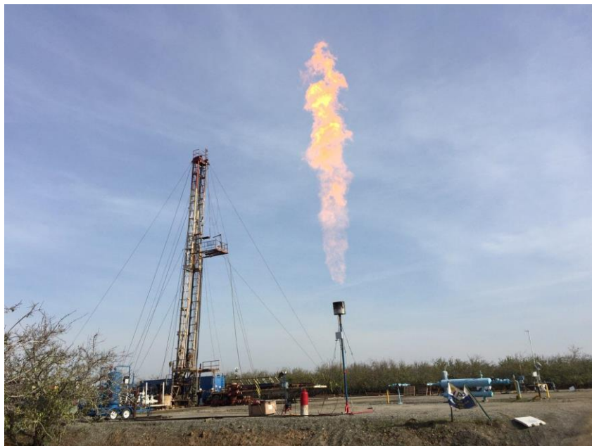
Historic Dempsey 1-15 Gas Flare before connection to sales pipeline
